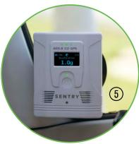
The feature-packed compact ADS-B and GPS receiver also offers a built-in carbon monoxide sensor with an alert system when carbon monoxide levels reach dangerous levels. Available in two variants: Sentry and Sentry Plus.
