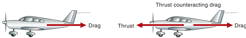
Figure 1-1 Drag counteracted by thrust.
