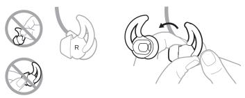
2. Align the opening of the new StayHear+ tip with the earbud nozzle and rotate the tip onto the nozzle. Press the base of the tip until it clicks securely into place.
